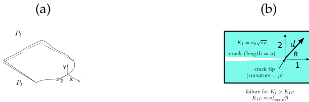
Figure 11.5: Cartesian (a) and polar (b) coordinate axes use d to define stresses in the vicinity of a crack tip.
