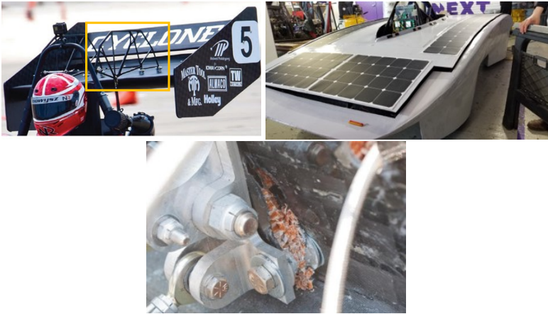
Figure 1: Carbon fiber integration into team vehicles. (a) Wing, (b) Aeroshell, (c) CF panel failure at bolt connection with suspension system..
