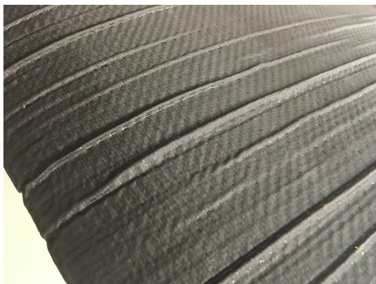
Figure 11: Dimples in a cured CF piece caused by poor placement of plies during the manufacturing process.
