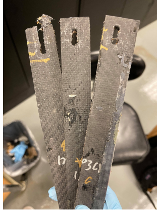
Figure 19: Bolt test parts after failure. Note the matrix failure localized to directly above the bolt.
