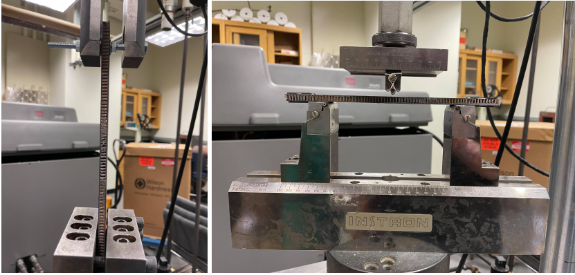
Figure 18: Mechanical testing methods employed. Bolt setup (left) and bend setup (right).
