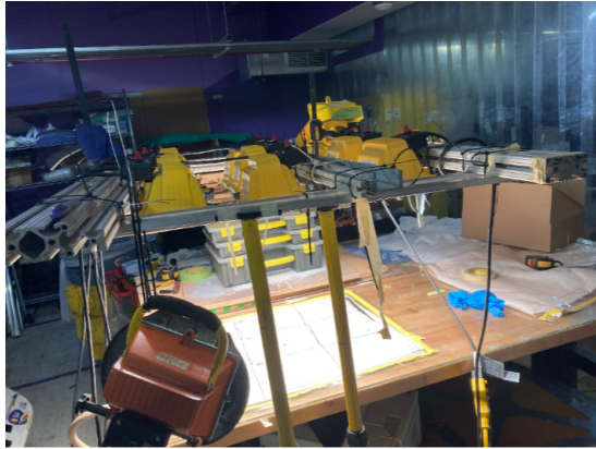
Figure 12: Lamp array setup used to cure our CF samples.
